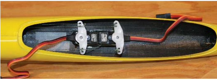
The radio compartment is generously sized, allowing you to position the gear for optimum balance. I will be moving the servos forward to reduce the need for ballast.
