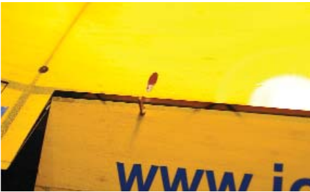
Hinging the ailerons on the lower surface allows a very low drag pushrod installation through the upper skin. Carefully mark and cut this hole to minimize its size.
