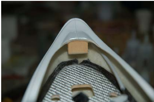
Glue Wood reinforcement 20mm x 20mm x 15mm
