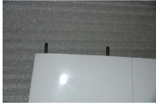
Glue the locating pins for te tips (3 mm dia carbon rods)
