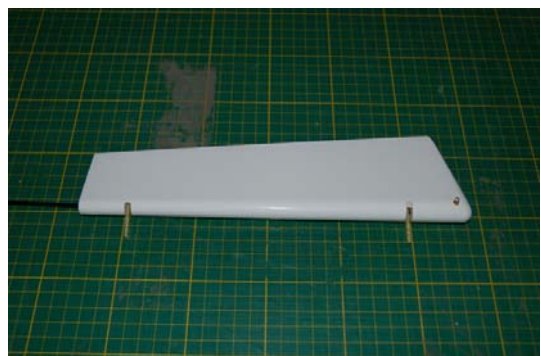
Glue hinges in place
