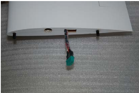
Glue the main wing locating pins in place (5 mm carbon rods)
