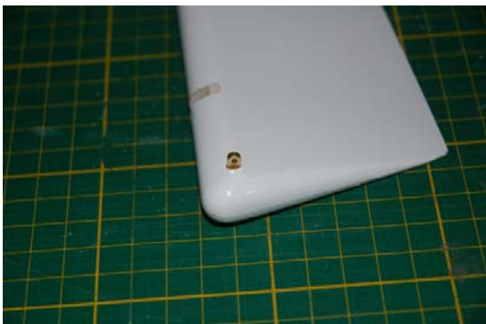
Install horn in rudder
