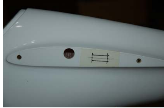
Make the holes for the servo connections
